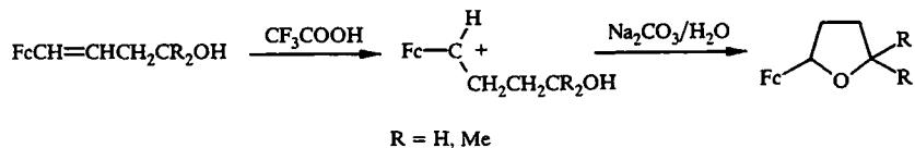
The most convenient and best studied method for the synthesis of 2-ferrocenyl- and 2,5-diferrocenyltetrahydrofurans is the cyclization of  $\gamma$ -glycols of the ferrocene series [41, 46-49]. The reaction takes place both in the presence of a dehydrating agent (10% sulfuric acid) [41, 49] and during vacuum distillation of the glycol [42-48] and gives a high and almost quantitative yield.
